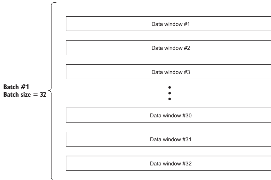
Figure 13.4 A batch is simply a collection of data windows that are used for training the deep learning model.
